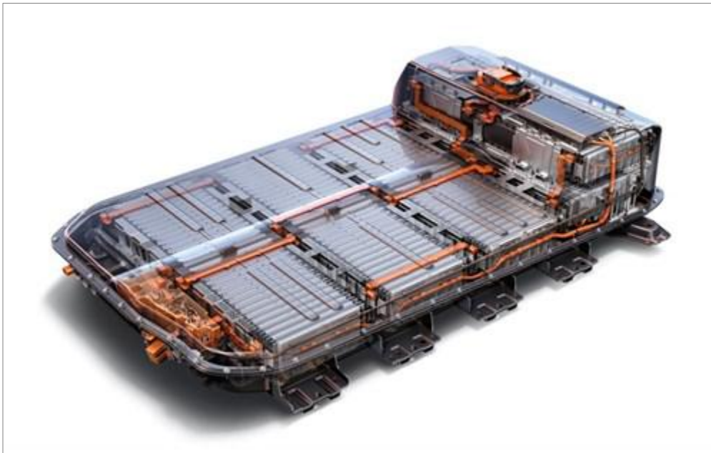
2017 Chevy Bolt 60 Kwhr Battery Pack
