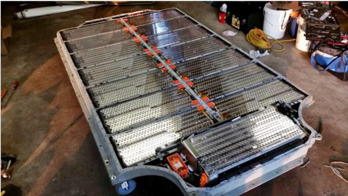
Tesla Model S 85 KWhr Battery Pack, with cover removed
