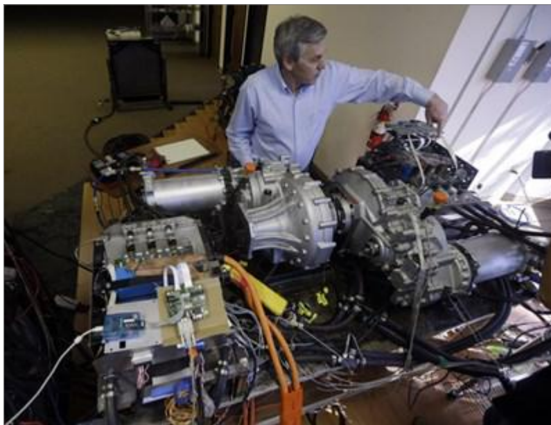
Ian Wright working on his turbine electric test bed
