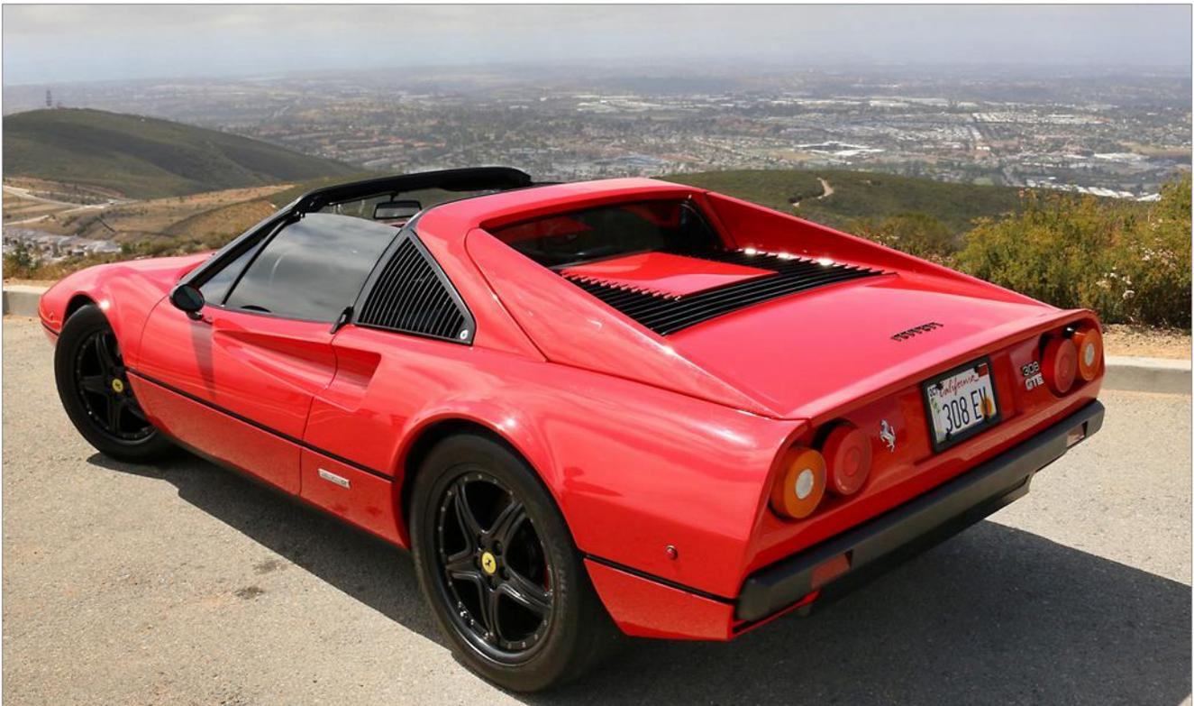
With three AC51 HPEVS electric motors and 48 batteries installed, the Cavallo Elettrico produces an impressive 465 horsepower and 330 pound-feet of torque. That's a heck of a lot more than the 2.9-liter V8 in the original 308 ever produced: before later versions introduced fuel injection and four-valve cylinder heads, the 308 packed about 200 horsepower and 181 lb-ft. Not one of the most powerful models ever to leave the factory in Maranello, in other words.
