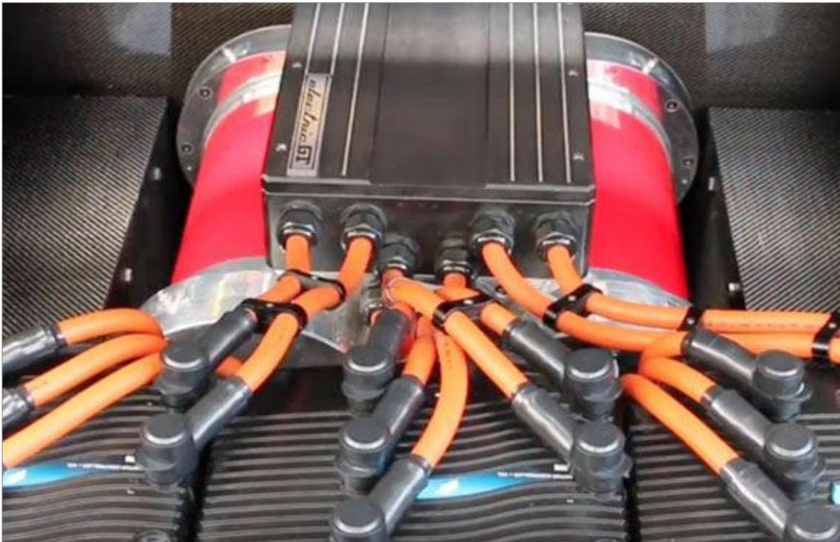
Three Controllers and Three AC51 Motors
