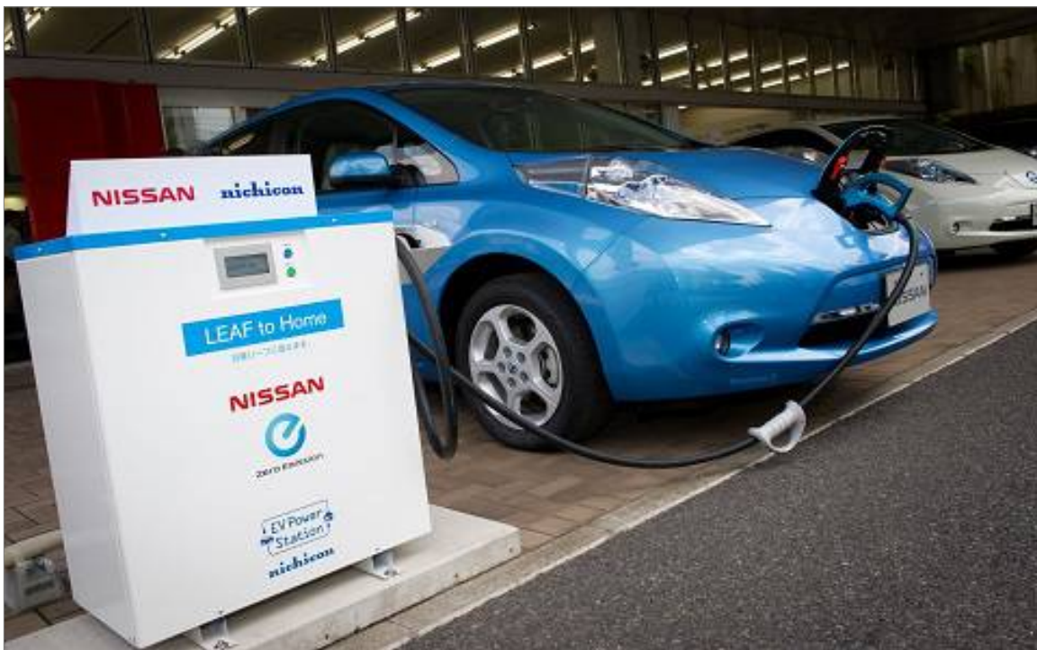
Nissan and Nichicon “Leaf to Home” system offered in Japan
