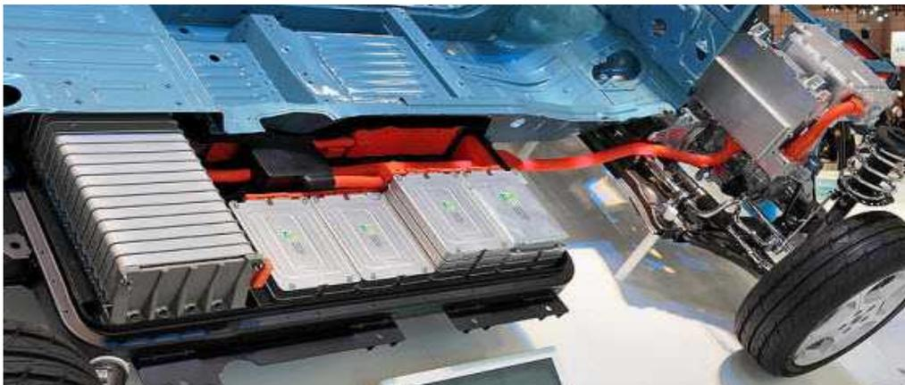
**Cut Away View of the Nissan Leaf 24 Kwh Battery Pack**
