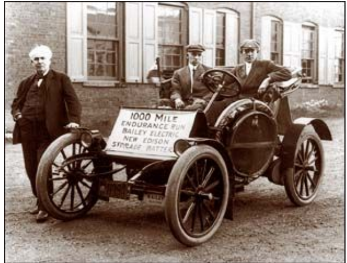
1910 – Edison’s 1,000 mile endurance test of his nickel iron alkaline battery using a Bailey Electric car. Edison and Ford planned to joint venture an electric car, but the electric starter was introduced in the 1912 Cadillac and in 1914 in Ford’s Model T. GM killed the electric car for the first time in the 20th Century.
