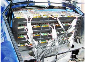
Joseph Gottlieb worked with Michael to build PC boards for controlling the voltage to each section of the lithium pack.
